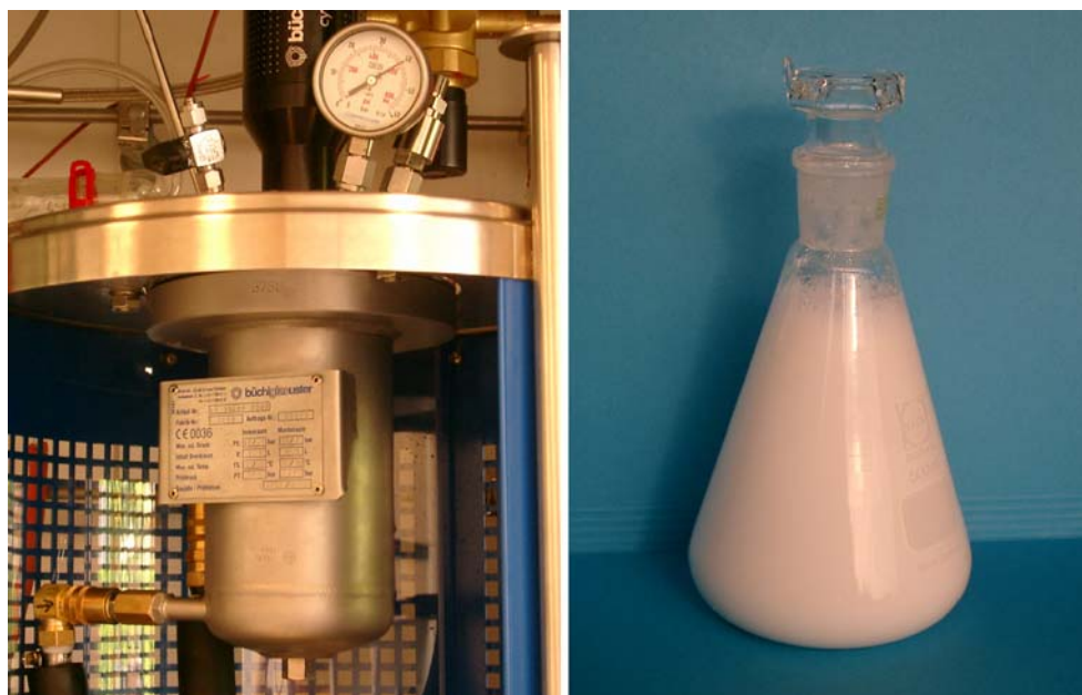
Fig. 1 Reactor utilized for catalytic emulsion polymerization ( left ) and polyethylene dispersion prepared ( right ; 0.5 l of dispersion with 10% solids content, M_n 10^5 g mol ^{-1} ; M_w/M_n 2.5; T_m 125 °C; catalyst productivity in dispersion synthesis 3 \times 10^4 TO over 2 h)
